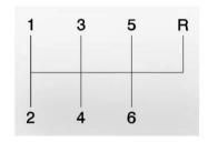
This is the shift pattern for the six-speed manual transmission.
